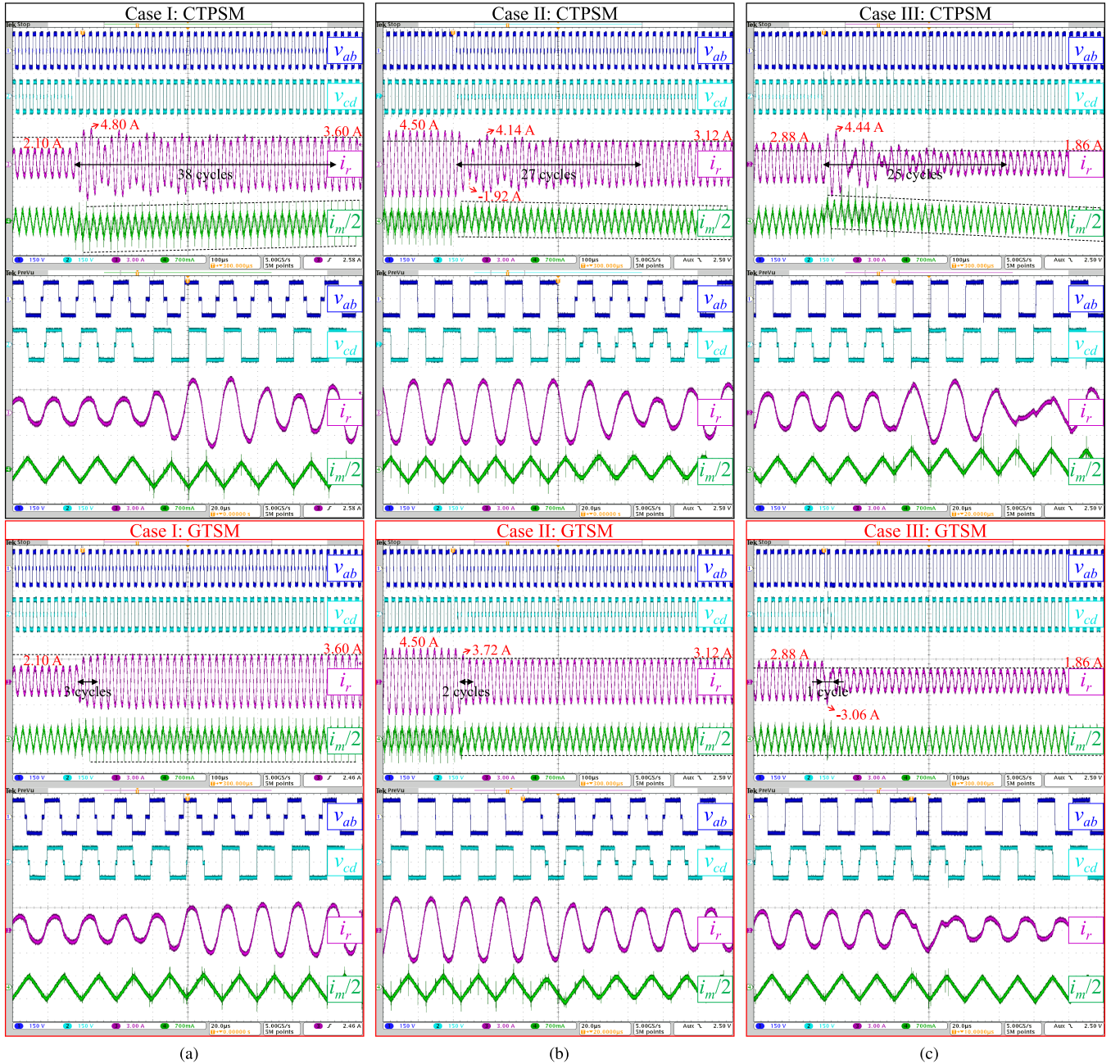
Fig. 11. Experimental open-loop transient waveforms with V_1 = 110 V, V_2 = 100 V, f_s = 50 kHz, and F = 1.2835 . (a) Case I: Increasing power accompanied by a transition from TPS mode to DPS mode (i.e., \theta_1 = 2\pi/15 , \theta_2 = 11\pi/60 , \theta_3 = \pi/10 , \Delta\theta_1 = \pi/15 , \Delta\theta_2 = 11\pi/60 , and \Delta\theta_3 = -\pi/10 ). (b) Case II: Decreasing power accompanied by a transition from SPS mode to TPS mode (i.e., \theta_1 = 0 , \theta_2 = 7\pi/15 , \theta_3 = 0 , \Delta\theta_1 = 2\pi/15 , \Delta\theta_2 = -\pi/6 , and \Delta\theta_3 = \pi/5 ). (c) Case III: Reversing power flow direction accompanied by a transition from DPS mode to SPS mode (i.e., \theta_1 = 0 , \theta_2 = \pi/4 , \theta_3 = \pi/10 , \Delta\theta_1 = 0 , \Delta\theta_2 = -23\pi/60 , and \Delta\theta_3 = -\pi/10 ).
